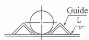
(F) Pipe support
