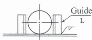
(E) Pipe support
